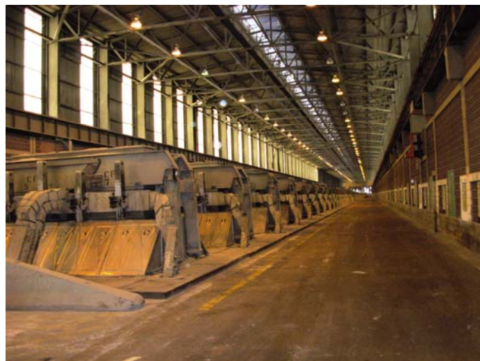
One of the smelter's six potrooms, which produce molten aluminium. Each potroom contains 140 electrolysis cells (pots)
